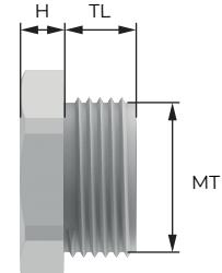
Thread Type **PG** acc. to DIN 40430
